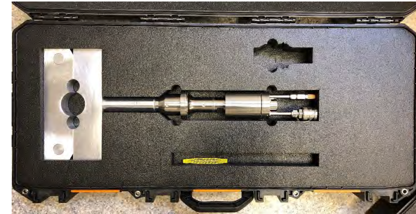
NU-DEC™ transducer clamp assembly (NPS 2" shown)
