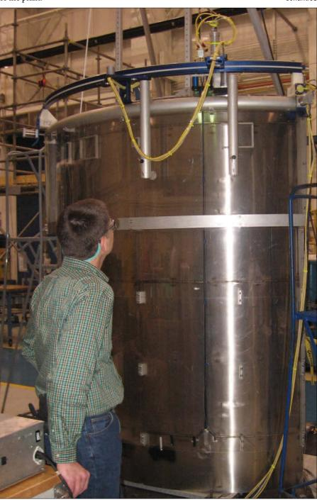
A fiberscope inspection tool was used at Point Beach to inspect the lower core barrel girth weld.
