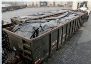
*Rail car liners for contaminated soils and construction debris meet the requirements for IP-1 containment.*
