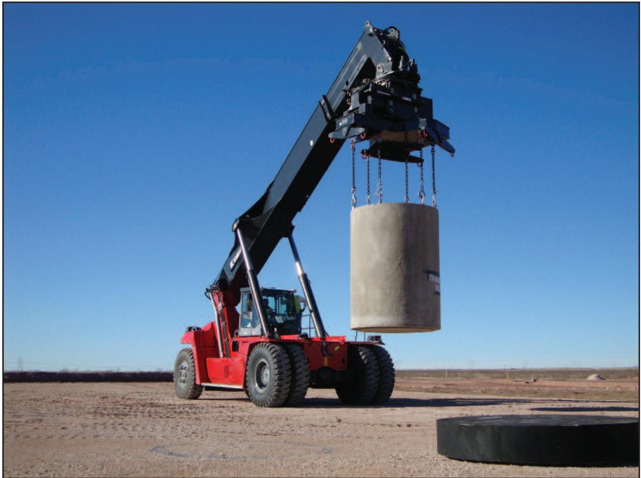
*Modified stacker (60-ton capacity) with modular concrete canister.*
