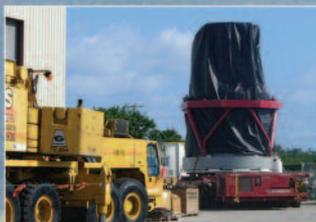
*These custom LSA and SCO over packs are being used in transport and are tested, project-proven, and meet IP-1 requirements.*
