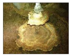
Salt deposits grow like mushrooms inside Hanford's single-shell storage tanks. An article beginning on page 32 compares the waste in Hanford tanks with that in Savannah River Site tanks.
