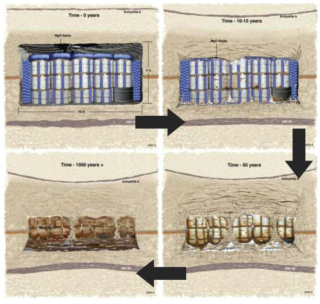
Fig. 5. Clockwise schematic illustration of the behavior of a disposal room in rock salt with time. As illustrated in the sequence, the rock salt will encapsulate the waste containers and close all void spaces, which, in turn, will prevent solids
