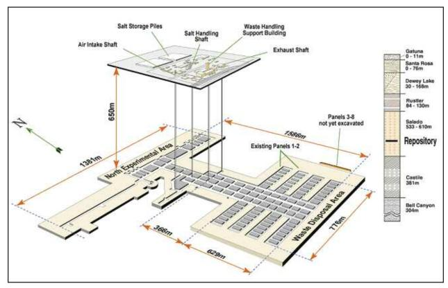
Fig. 1. Schematic illustration (not to scale) of the layout of surface and subsurface facilities and the stratigraphic column of the WIPP site. At the end of 2010, panels 1–4 (to the east) and 5 have been filled, panel 6 is being filled, panel 7 is being excavated, and panel 8 (opposite from panel 1) is to be excavated. Each panel has seven 4-m-high, 10-m-high,
