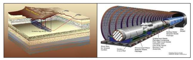
Fig. 2. Schematic illustration of the layouts of the Yucca Mountain HLW repository (in blue) and the underground re-
