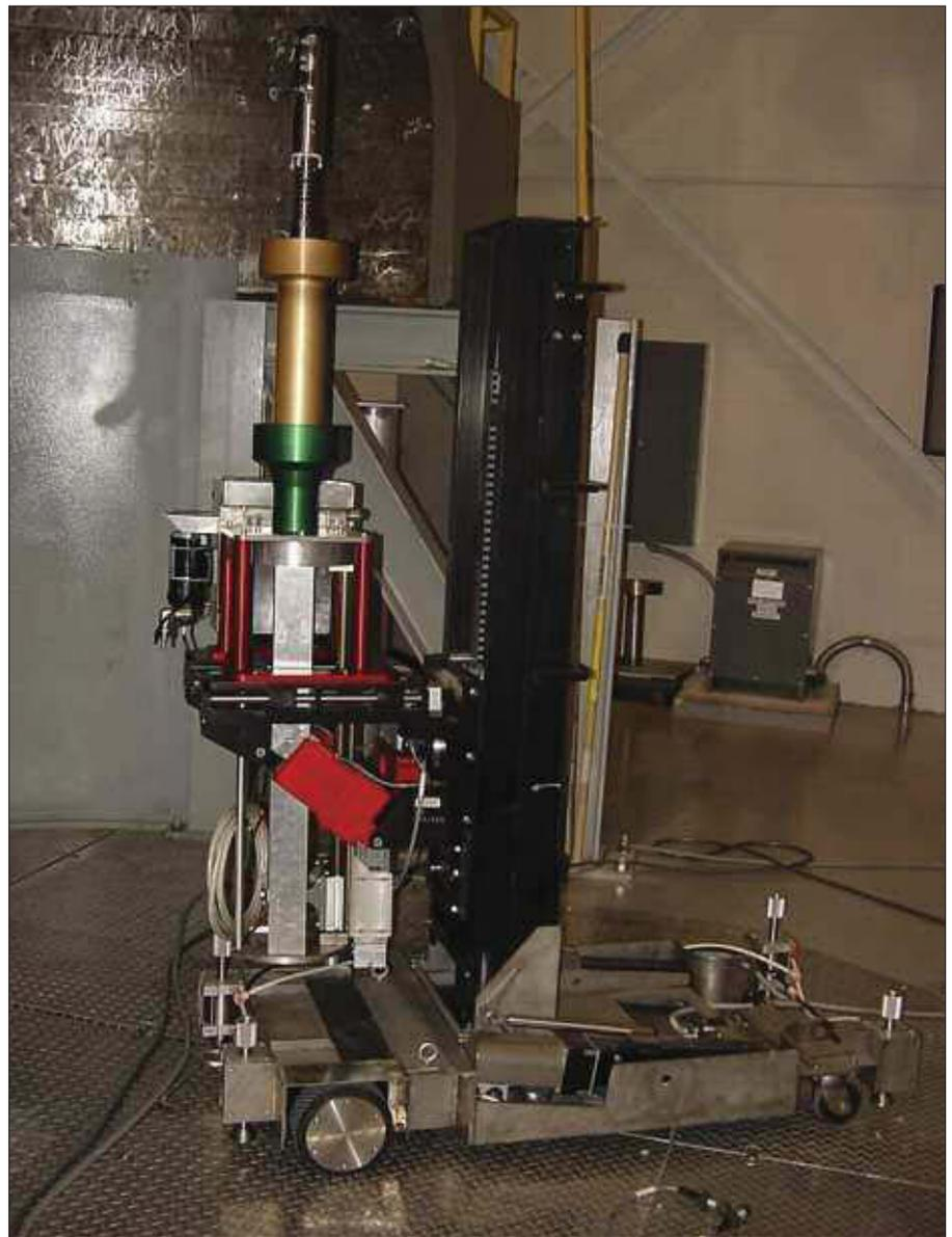
The development of an innovative device used to inspect reactor vessel heads won TIP's Best of the Best Award for employees at Entergy Nuclear's Palisades nuclear power plant. The gimballed head device, seen here on a delivery platform, uses ultrasonic transducers to identify irregularities within the welded steel vessel head nozzles used for control rod drive mechanisms and nuclear instrumentation. (Photos: NEI)
