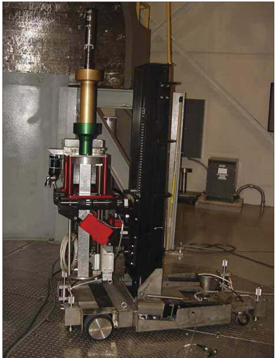
The development of an innovative device used to inspect reactor vessel heads won TIP's Best of the Best Award for employees at Entergy Nuclear's Palisades nuclear power plant. The gimbaled head device, seen here on a delivery platform, uses ultrasonic transducers to identify irregularities within the welded steel vessel head nozzles used for control rod drive mechanisms and nuclear instrumentation. (Photos: NEI)
