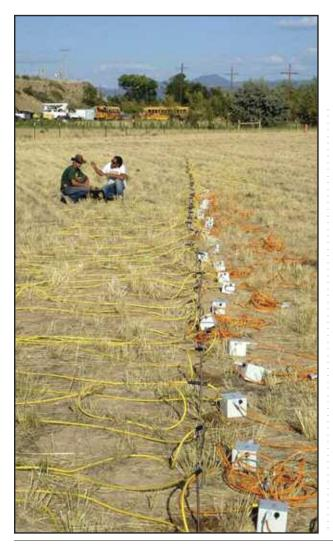
**Left:** Kenneth Williams, of Berkeley Lab, and graduate student Adrian Flores Orozco, of the University of Bonn, collect surface spectral-induced polarization at the Rifle Integrated Field Research Challenge Site. This work is helping to detect and delineate regions of naturally elevated subsurface microbial activity that could aid in halting the progress of radionuclides and other contaminants.
