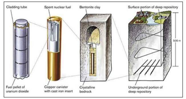
Fig. 4. Schematic illustration of the Swedish SKB-3V disposal concept (500 m = ~ 1640 ft). (Illustration courtesy of SKB.)
