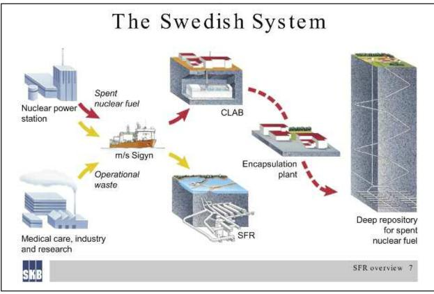
Fig. 1. Schematic illustration of core components of the Swedish nuclear waste management and disposal program/ system. (Illustration courtesy of SKB.)
