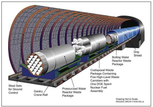
Fig. 3. Schematic illustration of the current disposal room design at the Yucca Mountain site.
