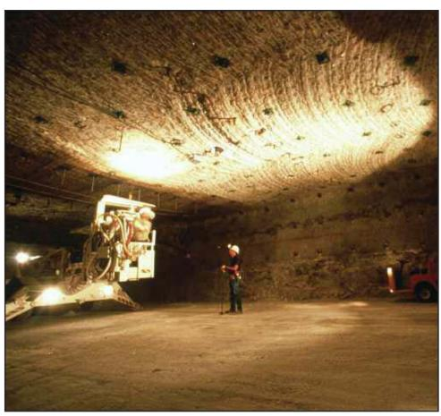
Roof bolting allows rooms to be maintained open and safe for as long as needed to complete emplacement operations.
