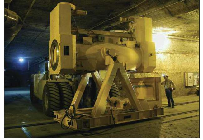
Large equipment underground, such as this facility cask shielding remote-handled waste in canisters, requires wide, tall openings underground.
