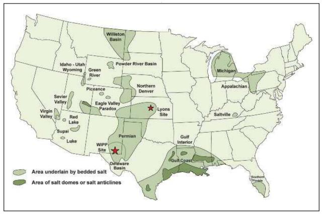
Deep geological salt deposits in the United States. The Delaware subbasin of the Permian Basin is the thickest contiguous deposit at a depth that balances closure rates with safe disposal operations.
