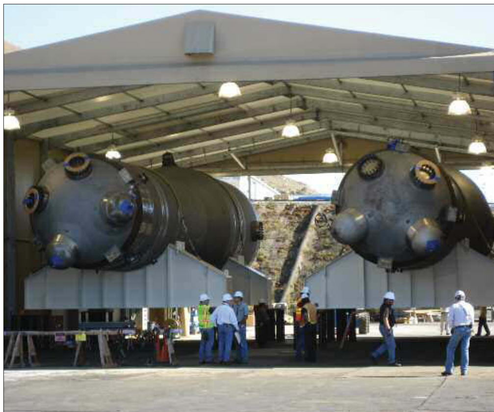
New steam generators in on-site temporary storage
