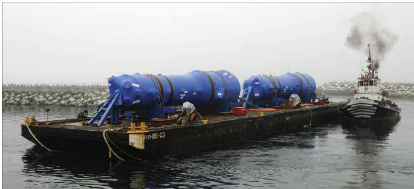
Two of the new steam generators arriving by barge at Diablo Canyon's intake cove (Photos: PG&E)
