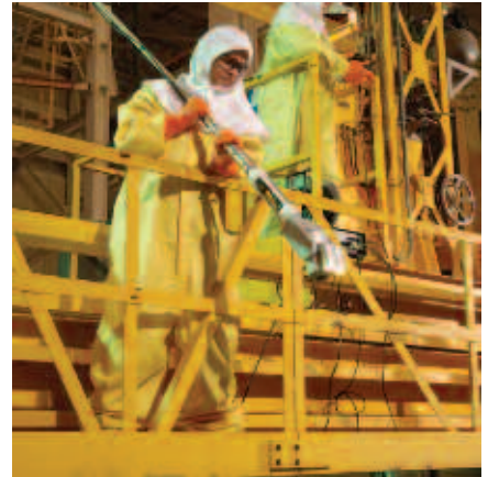
Operators perform nuclear reactor vessel visual inspection with Ca-Zoom PTZ Digital Inspection System
