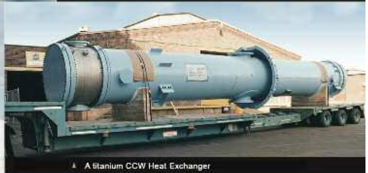
▲ A titanium CCW Heat Exchanger
