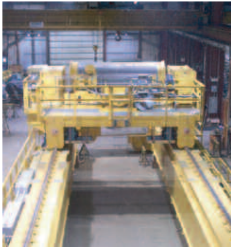
Complete 200 Ton Spent Fuel Handling Crane
