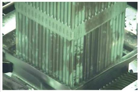
Visual inspection of a fuel assembly to assess crud loading
