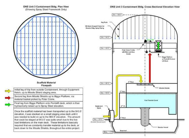
Illustrations showing the spray header steel grid (left) and a cross-sectional elevation view inside containment at Oconee
