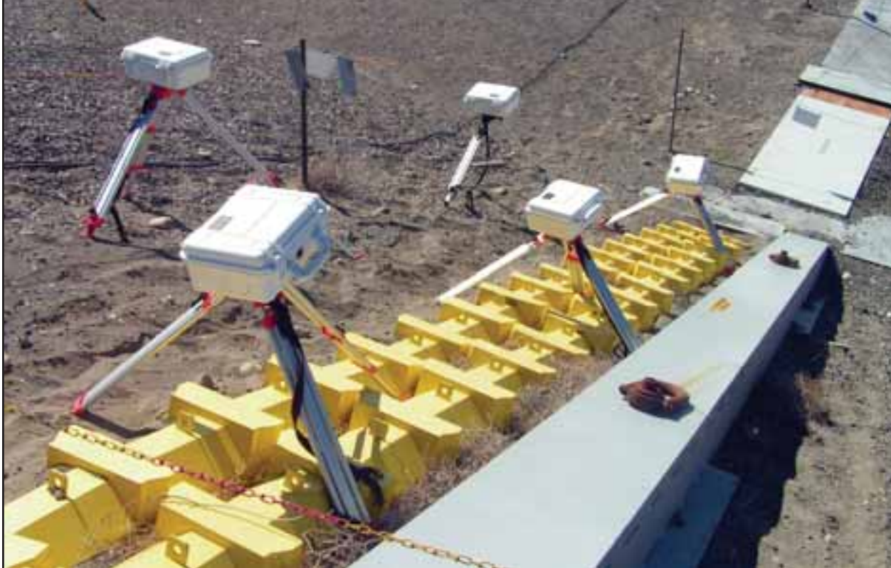
One of the newest applications of wireless technology is remote radiation monitors, which can be put in places where it would be dangerous to send workers.
