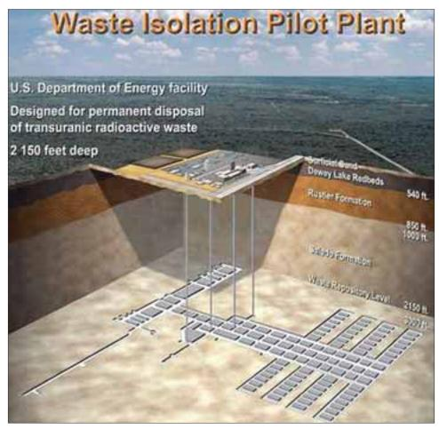
The Waste Isolation Pilot Plant, the only operating deep geologic nuclear waste repository
