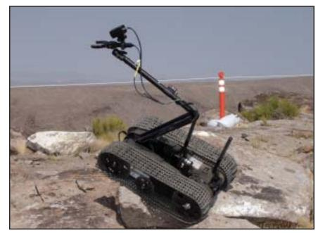
OCRWM is experimenting with new robotic technologies. Here, a robot, equipped with four video cameras and tank-like wheels, ascends a rock pile on the Yucca Mountain crest.
