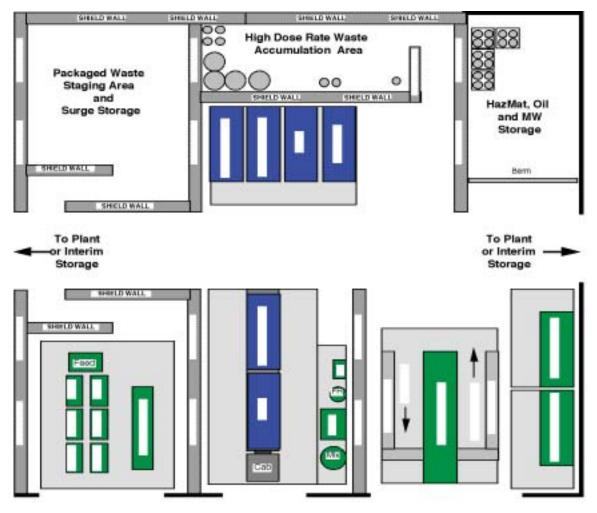
Fig. 4. Potential configuration for an idealized mobile treatment system facility for new plants.
