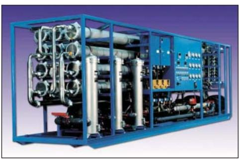
Fig. 3. Typical power plant reverse-osmosis mobile processing unit.
