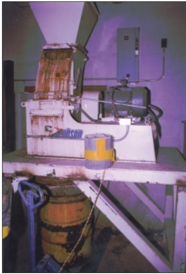
*(Left) Loading scintillation vials into the vial crusher's bin. Liquid is drained into the bottle at the lower right, and the crushed glass and plastic go into a separate drum. (Right) The old vial crusher could only be used by climbing a ladder to dump vials into the funnel. This unit is now in the process of being decontaminated and removed for disposal.*
