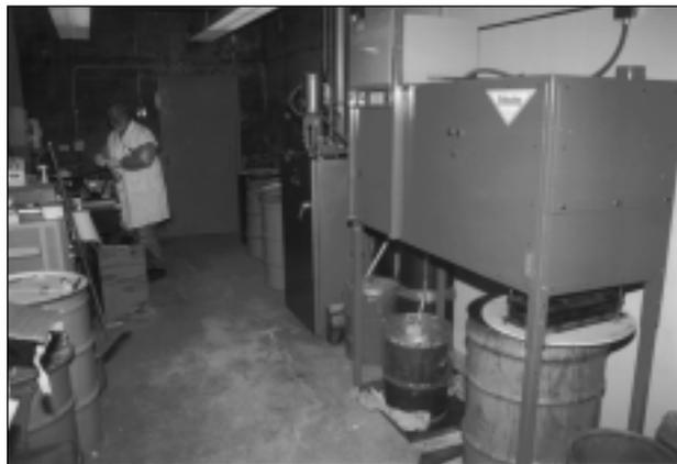
*University of Rochester LLRW processing room. In the foreground is the vial crusher with the waste compactor just past it. Technician Chuck Surre is wearing his protective equipment—a lab coat, gloves, safety glasses, and plastic sleeves. Extensive air sampling has never shown evidence of airborne radioactivity*
