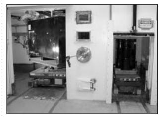
The waste packaging system allows for bagless transfer of wastes from boxes and drums through these ports, shown during testing.
