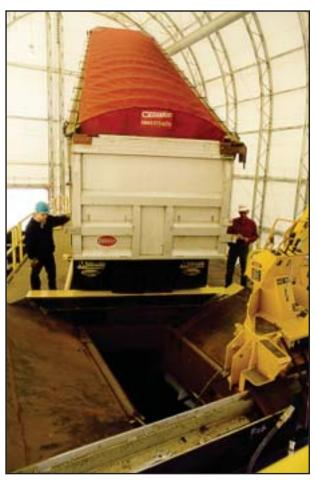
Bulk materials inside MHF Logistical Solutions' totally enclosed transload facility in Worcester, Mass., being transloaded from a truck to a gondola railcar, positioned below, for shipment by rail.
