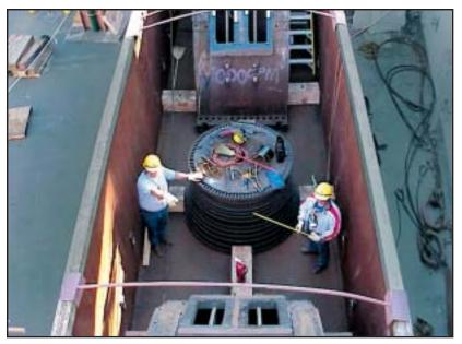
Turbine rotor blades from San Onofre-1 being transported in a high-sided gondola railcar.
