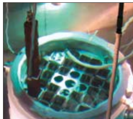
Loading a fuel bundle into a spent fuel storage cask at Big Rock Point. The photo essay beginning on page 32 looks at how the plant became fuel free.
