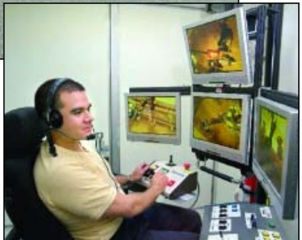
*Surrounded by a bank of viewing screens, an operator uses joysticks to control dexterous movements by the Pit Viper robotic arm.*
