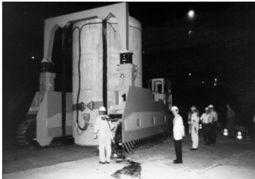
An empty VCS container is moved to the reactor building to be loaded with spent
