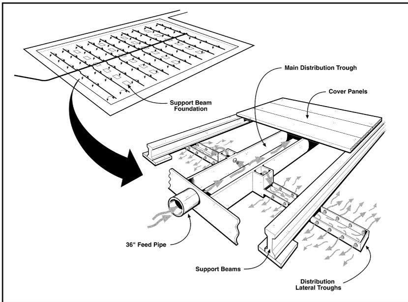
N Reactor cooling water was released to the soil through cribs. The water entered the 116-N-3 crib through a 36-in. feed pipe and was distributed over 1.3 acres of soil via a central distribution trough and a series of lateral troughs.
