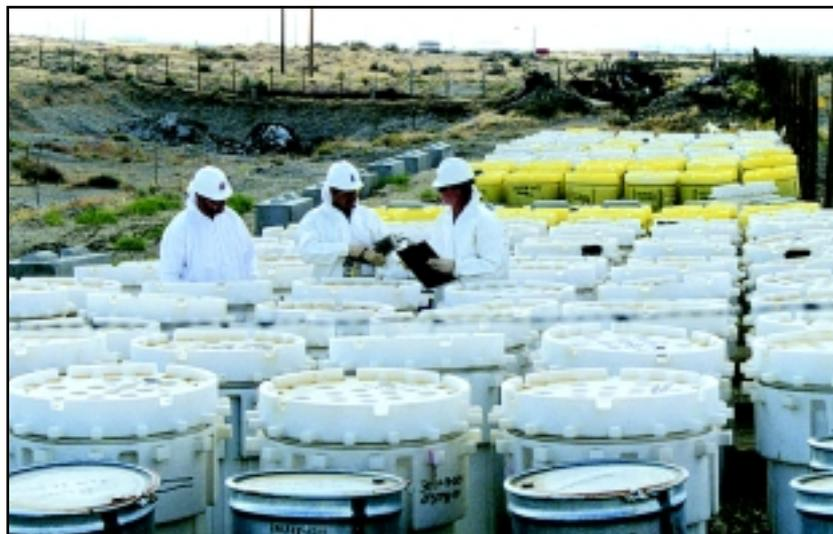
*Twice a month, Bechtel Hanford waste transportation specialists and radiological control technicians monitor 338 drums containing uranium oxide or depleted uranium shavings covered in oil. The barrels were discovered at the 618-4 Burial Ground north of Hanford's 300 Area in 1998. Project staff are developing a plan for the safe disposal of about 1200 more barrels that they believe are buried at the site.*
