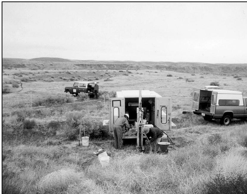
*Field personnel push geoprobe rods into the soil before performing gamma-ray logging. The Environmental Restoration Project team avoided nearly \$20 million in cleanup costs by using the system to distinguish between natural and man-made gamma-emitting materials in the soil.*
