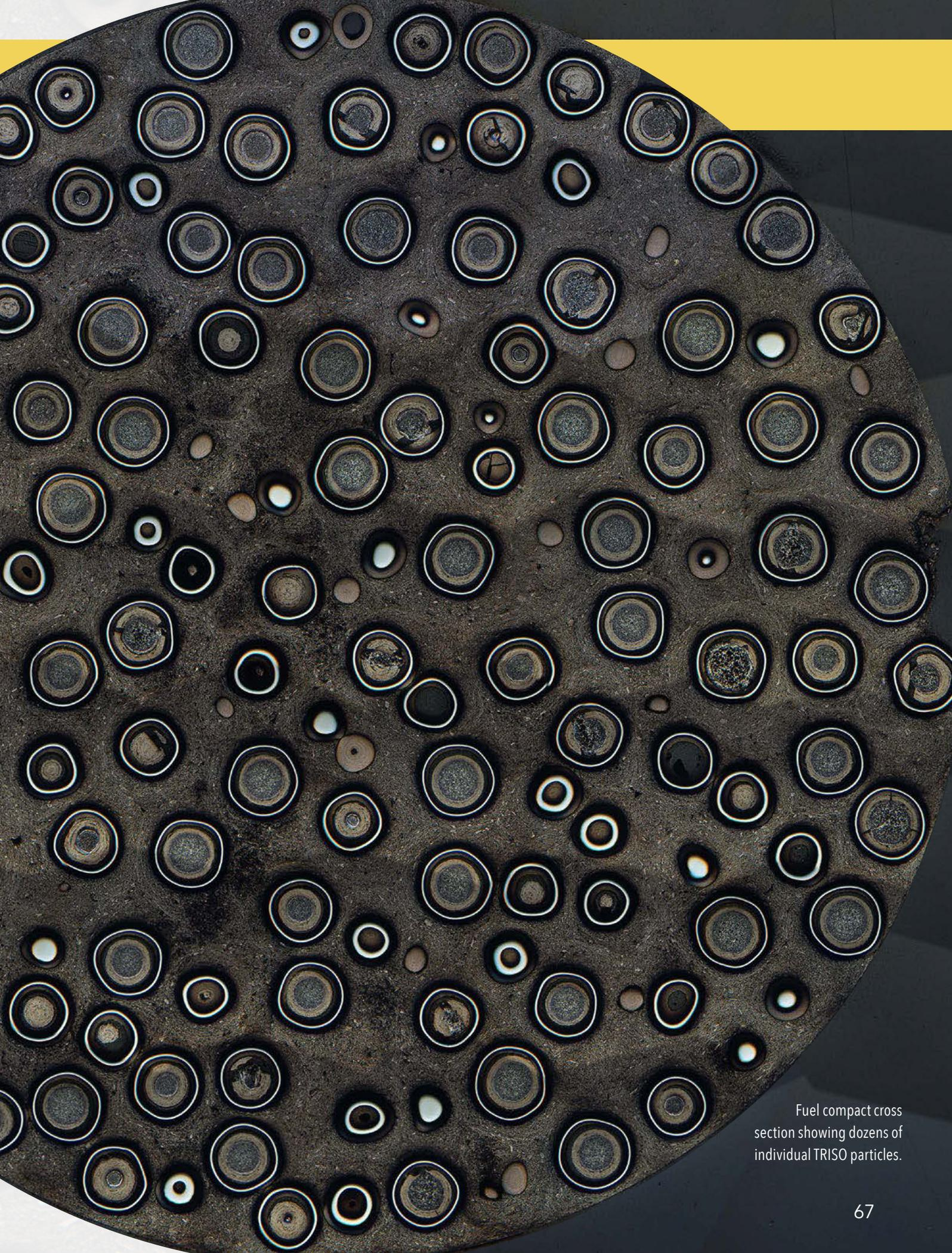
Fuel compact cross section showing dozens of individual TRISO particles.
