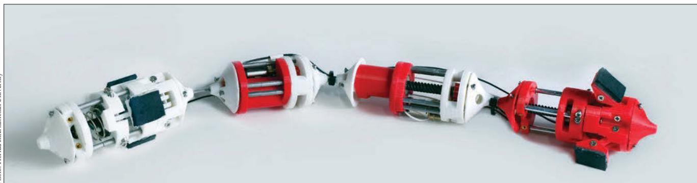
**Fig. 4:** Prototype of FIU's 2-inch crawler.
