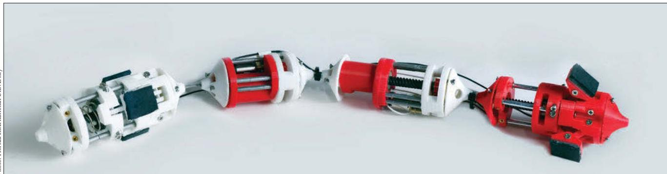
**Fig. 4:** Prototype of FIU's 2-inch crawler.
