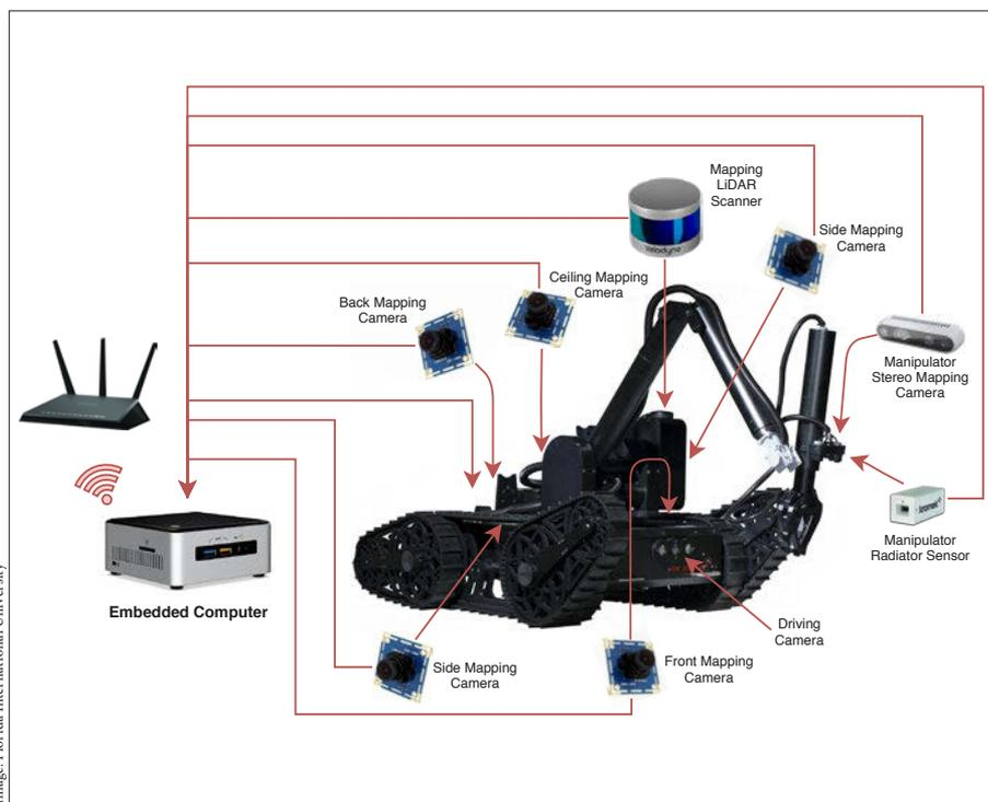
**Fig. 9:** The Jaguar V6 tracked robotic platform with arm manipulator and instrumentation.
