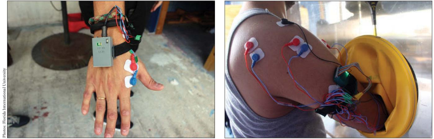
**Fig. 6:** Electromyography sensor for human testing, placed on the hand and arm.
