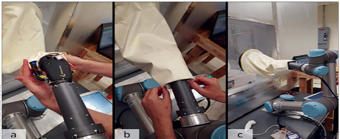
**Fig. 7:** Procedure for inserting the hand into the glovebox for testing: (a) initial hand posture to insert fingertips into the glove, (b) hand fully inserted into the glove, and (c) the arm inserting the hand into the glovebox.
