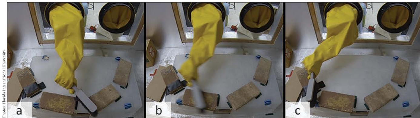
**Fig. 8:** Photo sequence of the brick-brushing task during the motion of one brushing stroke.
