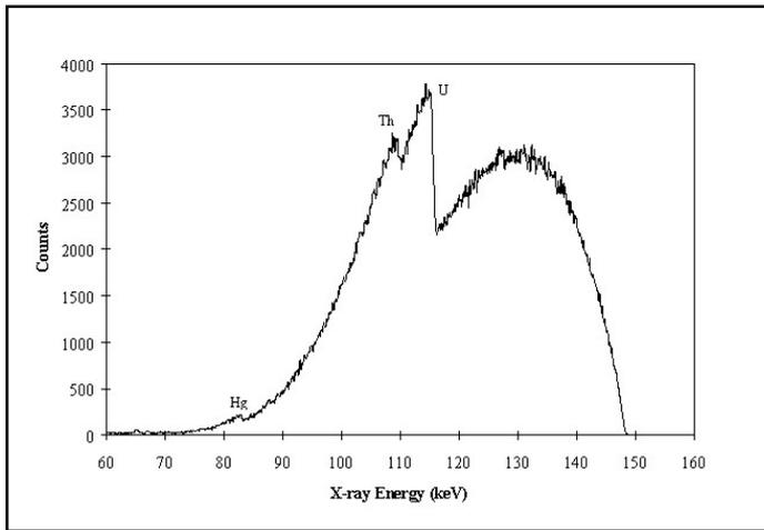
▲ Fig. 3. A chart of the X-ray, K-edge energy spectrum of mercury, thorium, and uranium contamination taken inside a drainpipe. The Portable X-Ray, K-Edge Heavy Metal Detector makes possible the detection of radionuclides within pipes and equipment without having to cut into them. This assay system improves worker safety by revealing internal contamination and locating the best areas to dismantle pipes and equipment. (TechID 134)
