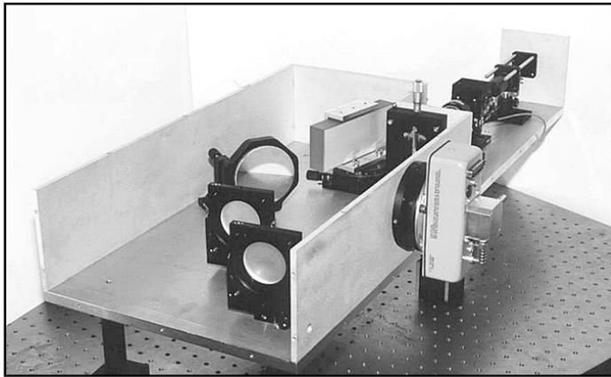
▲ Fig. 5. The Compact High Resolution Spectrometer is a versatile optical spectrometer for use in field and process applications. This real-time monitor can analyze actinides and continuously monitor EPA-regulated toxic metals, uranium isotopes, and actinides in stack gases. Cost savings result from on-line process control and reducing the need for intensive front-end waste characterization. (TechID 1564)
