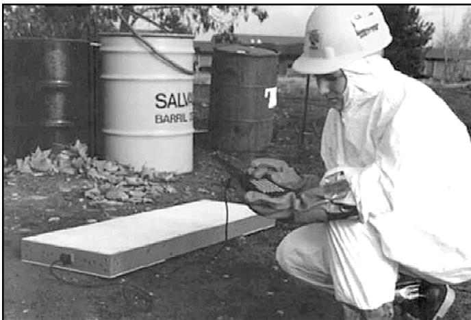
Fig. 4. The BetaScint™ Fiber-Optic Sensor minimizes costly sampling and analysis by allowing a technician to locate strontium-90 and uranium-238 on soils and pavements. The conventional method obtains samples for later offsite laboratory analysis. This sensor reveals the presence of beta emitters in real time, resulting in cost and scheduling benefits. (TechID 70)
