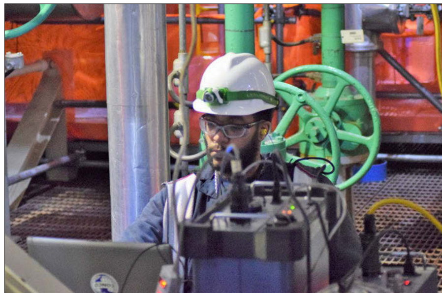
A Conco employee conducts feedwater eddy current testing during the outage.
