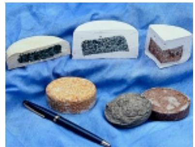
A revolutionary family of silicone-based geopolymers that can coat or encapsulate waste, facility surfaces or equipment
