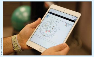
The Digital Plant Viewer is a Web-based application that provides an interactive plant map with 360-degree images, live video, real-time radiological exposure data, and wireless telemetry.
