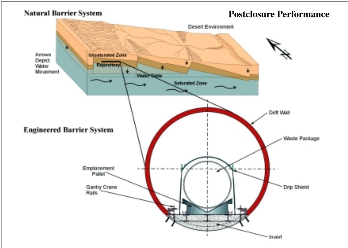
Fig. 3. A geologic repository at Yucca Mountain would rely on the area's dry climate as well as the natural and engineered barriers to contain and isolate the waste for thousands of years.
