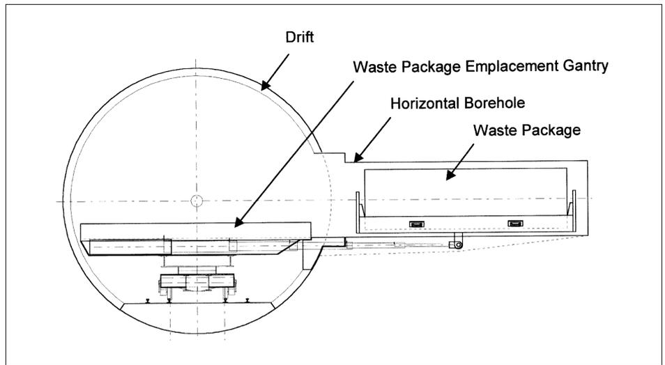
Fig. 5. Another version of the borehole concept called for placing the waste containers in holes drilled into the sides of the walls of the emplacement drifts.
