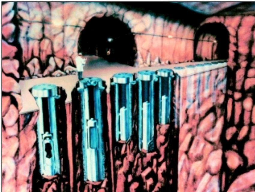
Fig. 4. The early design for the repository envisioned the waste containers being stored in vertical holes, with each hole accommodating a single canister and a closure plug providing some shielding against radiation.
