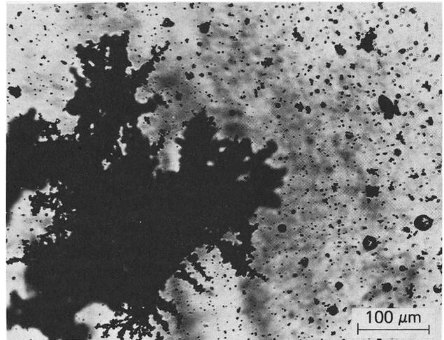
Fig. 3. Aerosol collected from HTCA Test 13 showing a bimodal aerosol distribution (Ref. 12).
