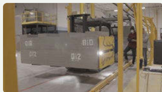
A modified forklift with a customized handling attachment is used to move spent fuel containers and their heavy bentonite clay housings. (Photo: NWMO)
