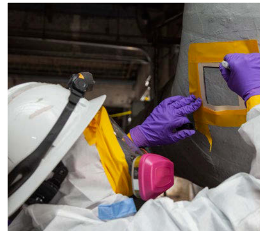
(Above) A worker takes samples inside Alpha-2 to characterize any risks and hazards in the building so that EM can safely plan and perform deactivation efforts.
