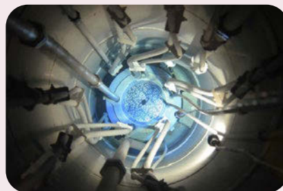
The core of SLOWPOKE-2. (Photo: CNL)
