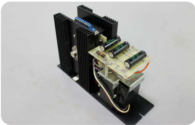
Power supply with electrolytic capacitors provided for repair by Duke, Westinghouse P/N: 475031 120VAC input +/-15V and -22V output. Another good candidate for parts quality testing.
