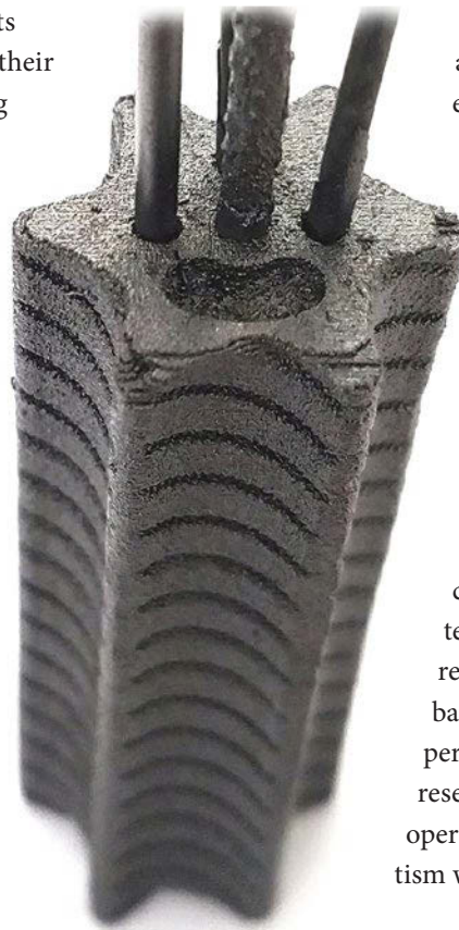
Fig. 4. Four embedded sensors in a 3D-printed silicon carbide structure.
