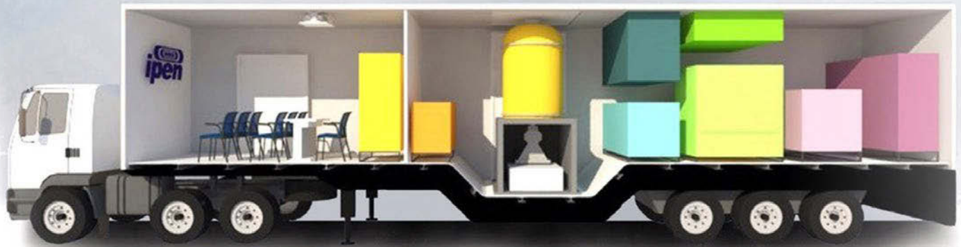
A cutaway illustration of Brazil's mobile electron beam unit.
