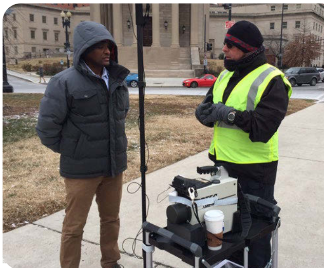
Trombino (right) demonstrates the RaFTS device with a high-purity germanium detector. (Photo: LLNL)
