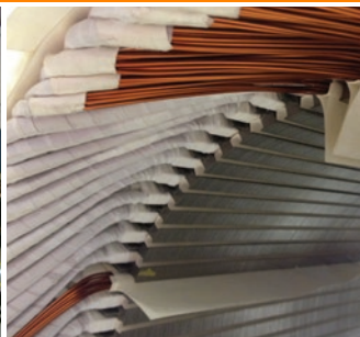
NUREG-0588 CAT-I (EQ) Insulation Systems
