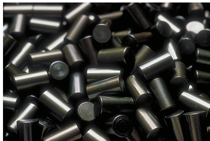
Figure 1. Unirradiated UO 2 fuel pellets before being inserted into the fuel cladding.
