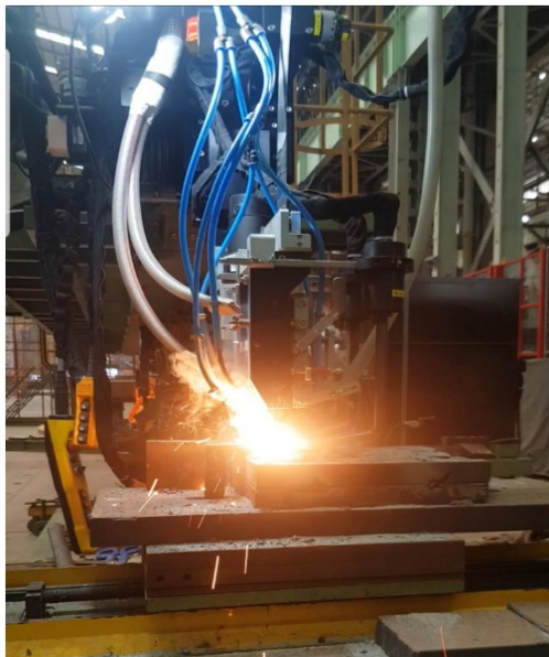
Automated cladding machine at Doosan
