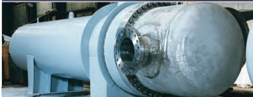
A 316 stainless RHR Heat Exchanger ▲
