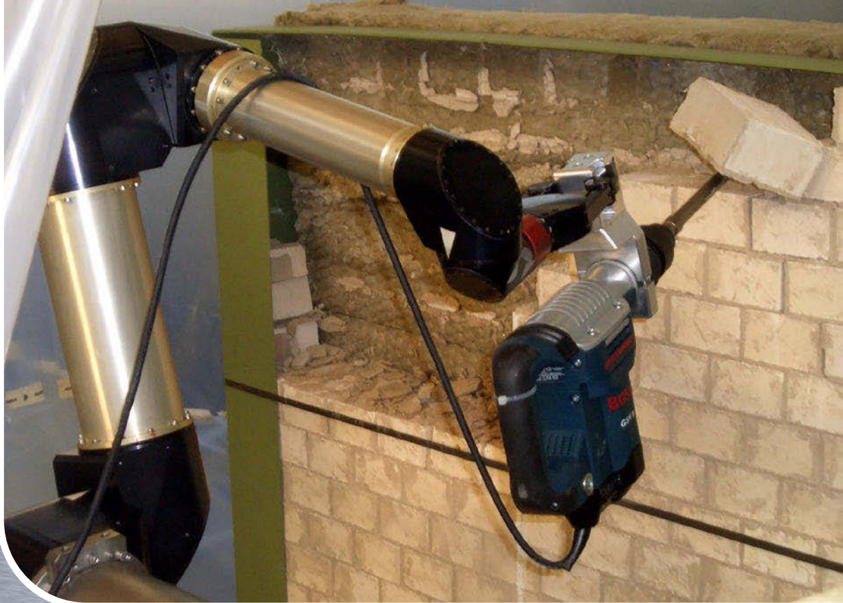
A Wälischmiller Telbot is used for decommissioning work.
