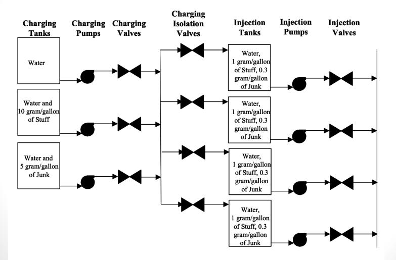
Figure 3. Fluid Injection System Schematic
