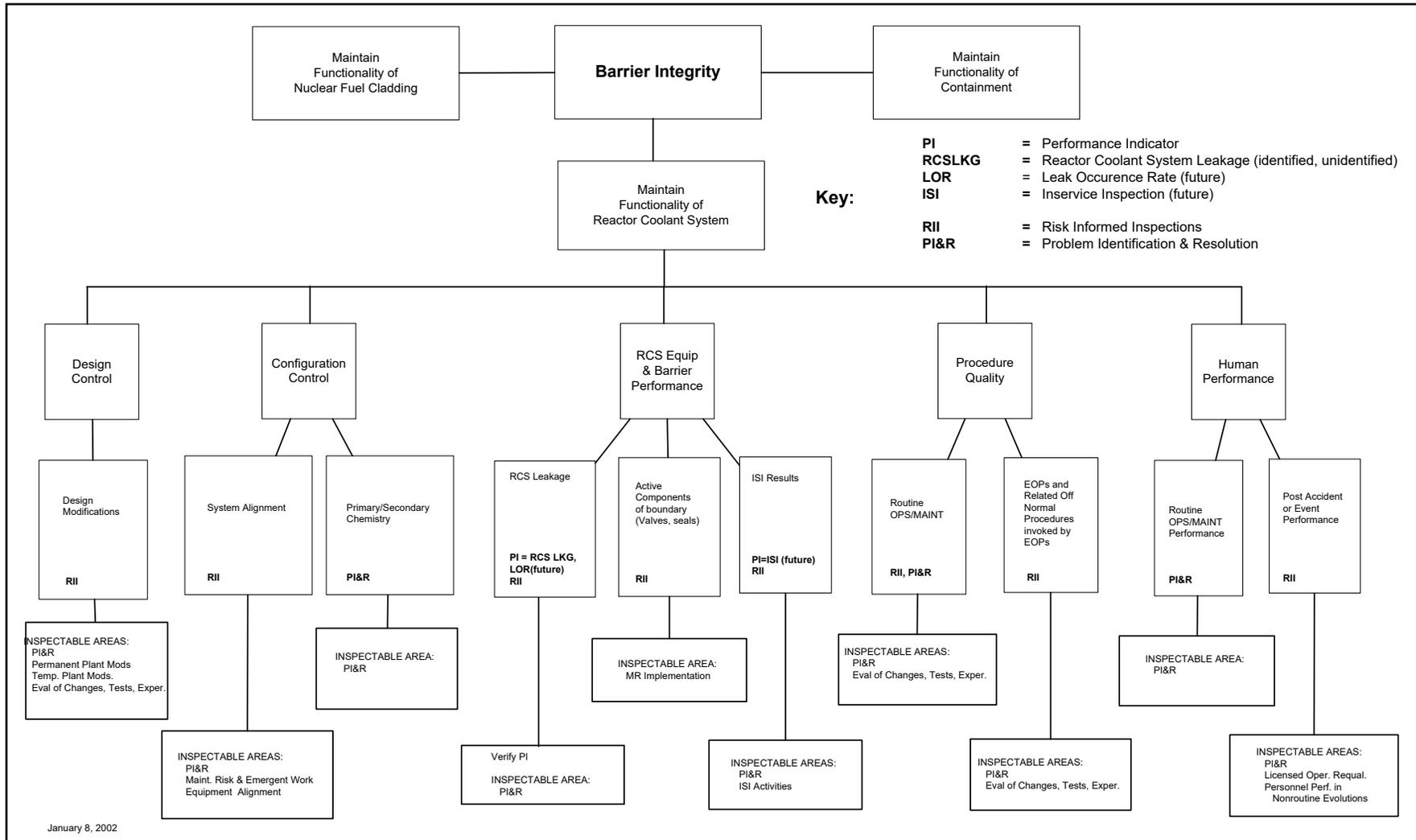
Figure 8. Performance Factors for Reactor Coolant Pressure Boundary (Barrier Integrity Cornerstone)
