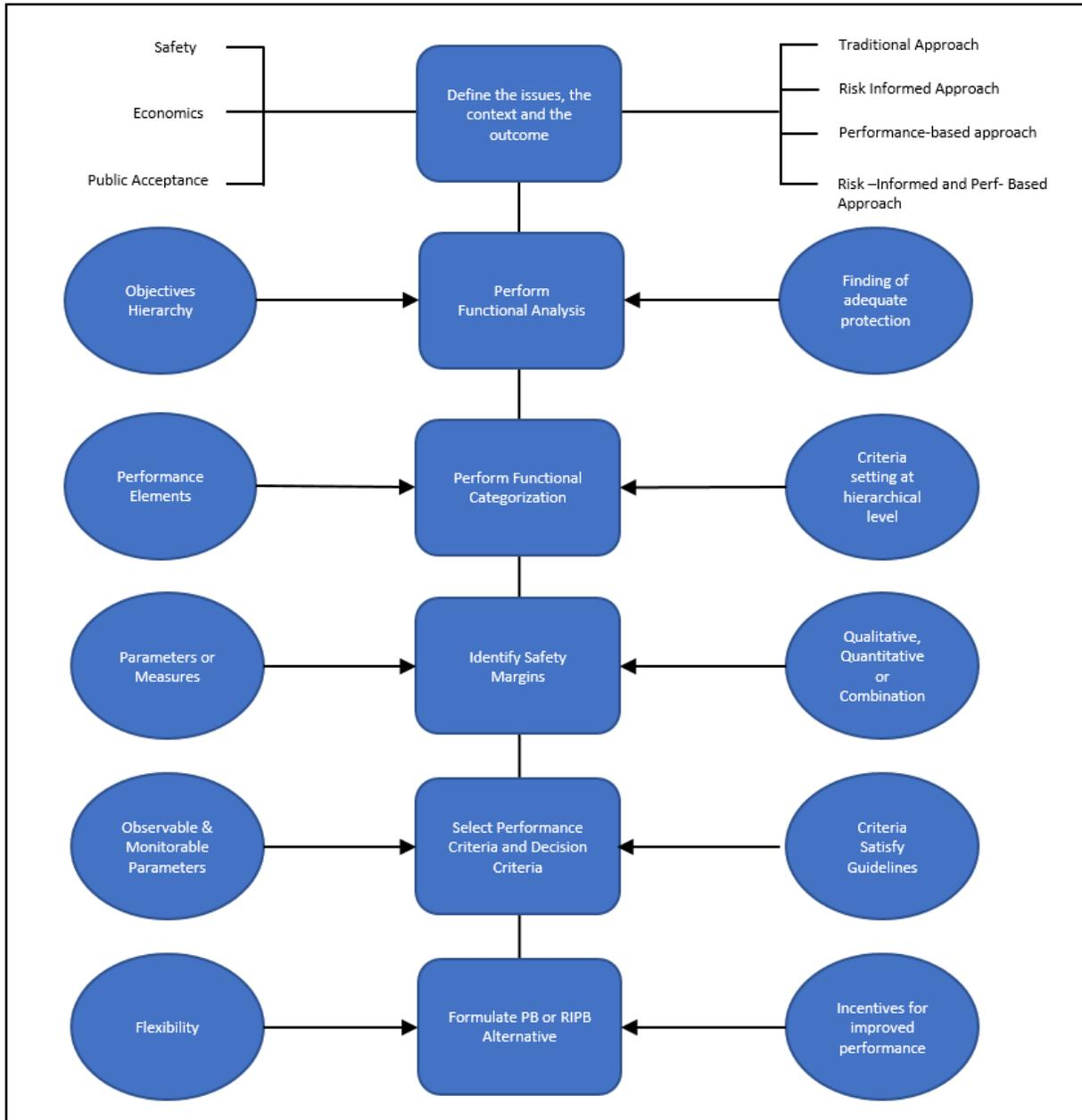
Figure 4. Implementation Steps for Performance-Based Approach
