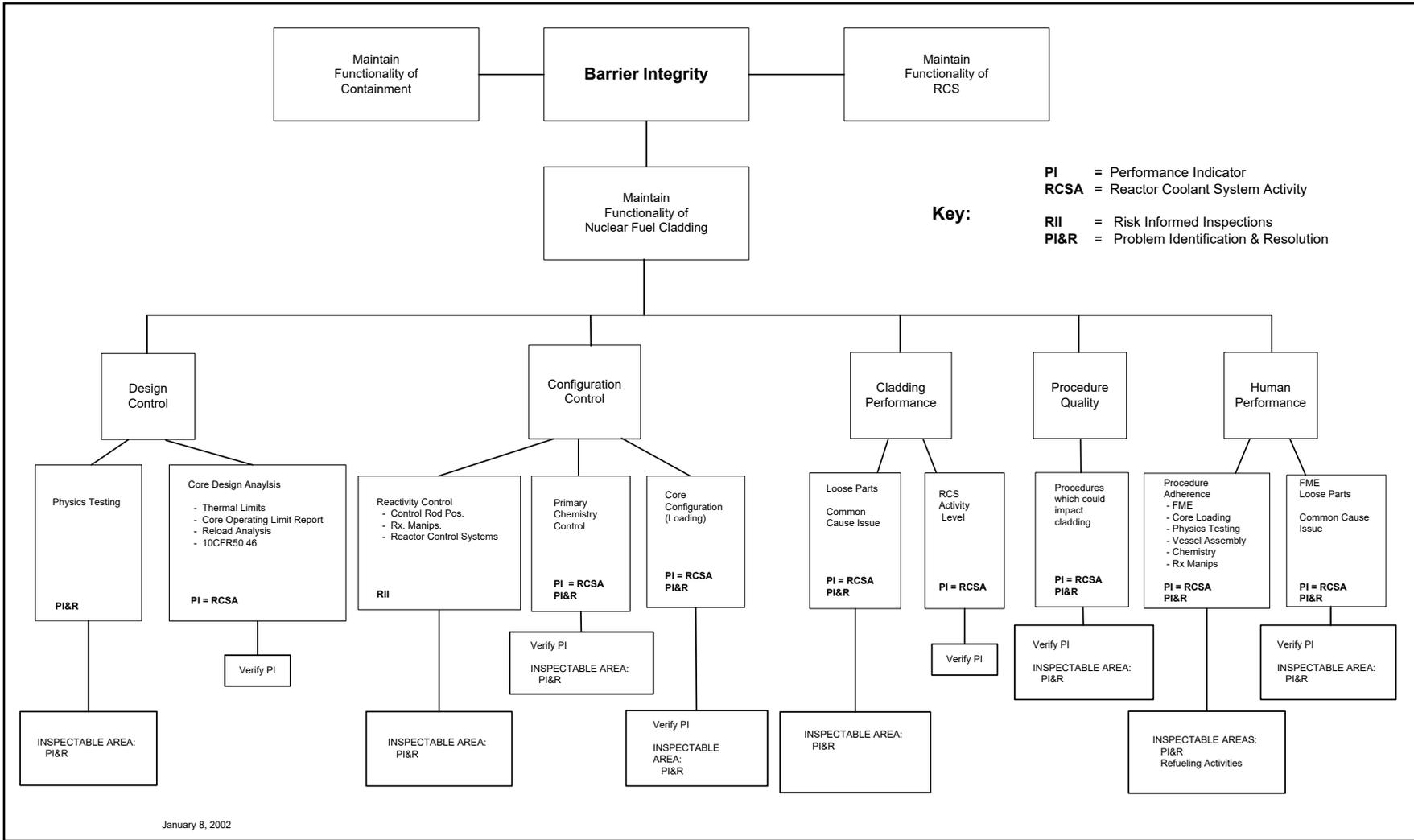
Figure 7. Performance Factors for Fuel Cladding (Barrier Integrity Cornerstone)
