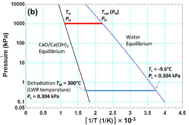
Fig. 1: Schematics of (a) components of a CHP system and (b) a heat pump cycle on the Clausius-Clapeyron diagram showing equilibrium of CaO/Ca(OH)<sub>2</sub> and H<sub>2</sub>O(L)/H<sub>2</sub>O(G).
