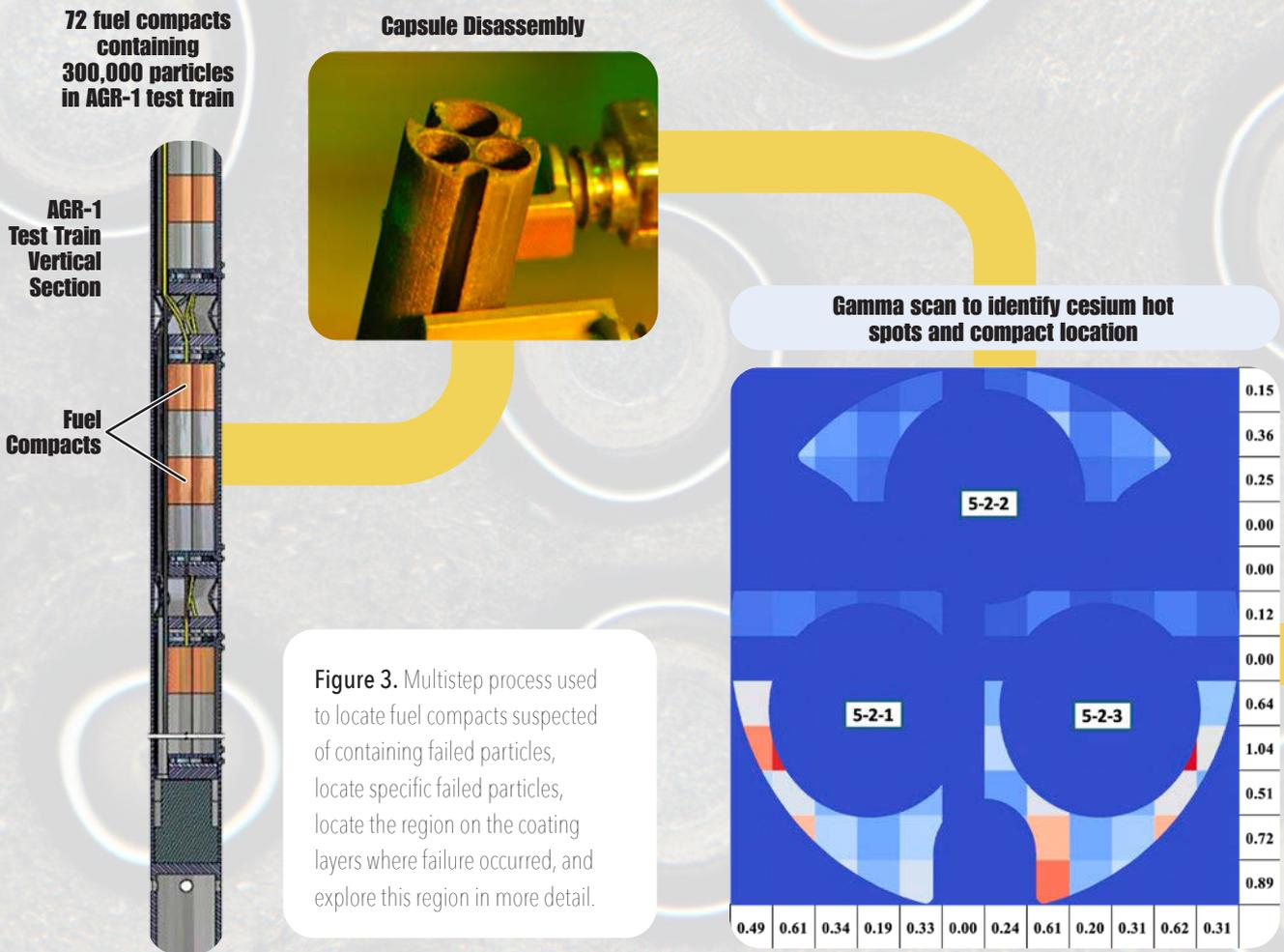
pects has been obtained from the AGR-1 and -2 irradiation and PIE campaigns. TRISO failure rates during irradiation were determined primarily by R/B data, as discussed above. Where fission gas release data during irradiation were inconclusive, additional information from PIE was used to help evaluate TRISO failure rates.
