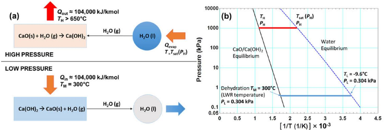
Fig. 1: Schematics of (a) components of a CHP system and (b) a heat pump cycle on the Clausius-Clapeyron diagram showing equilibrium of  $\text{CaO/Ca(OH)}_2$  and  $\text{H}_2\text{O(l)/H}_2\text{O(g)}$ .
