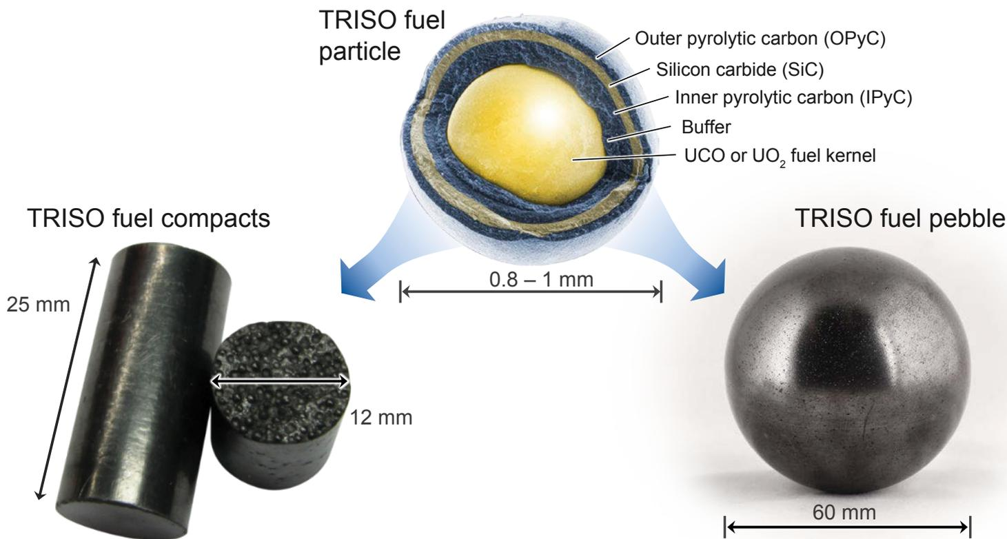
**Figure 1.** TRISO fuel particle, fuel compacts, and spherical fuel pebble. Fuel pebble image provided by X-energy LLC.
