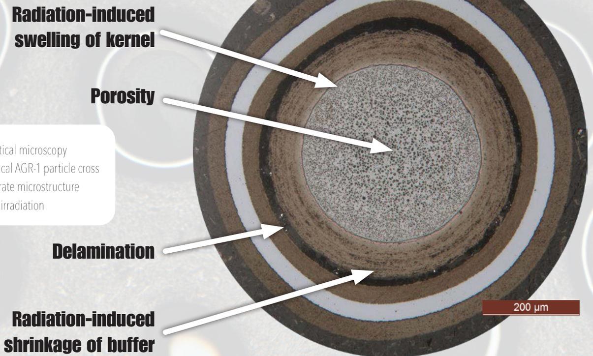
Figure 5. Optical microscopy images of typical AGR-1 particle cross sections illustrate microstructure changes after irradiation
