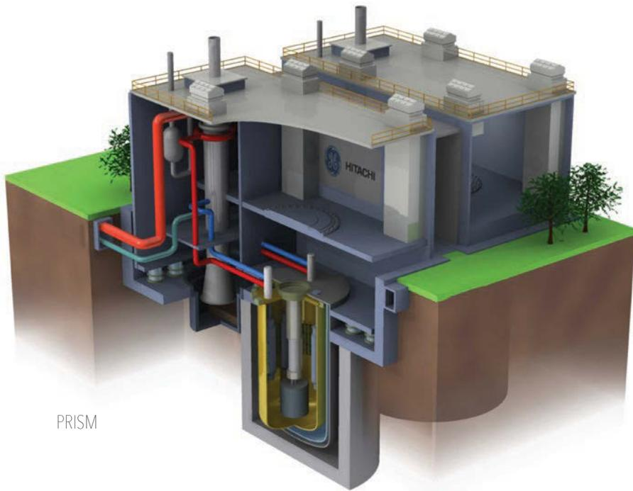
After the cancellation of the CRBR, the DOE funded the development of several liquid metal-cooled reactor designs. The most developed of these were SAFR (canceled following the development of conceptual design and partial review by the NRC) and PRISM.
