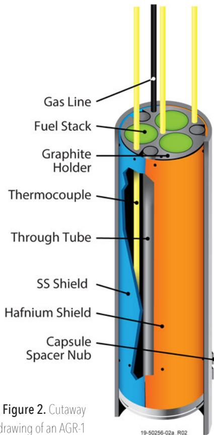
Figure 2. Cutaway drawing of an AGR-1 irradiation capsule.
