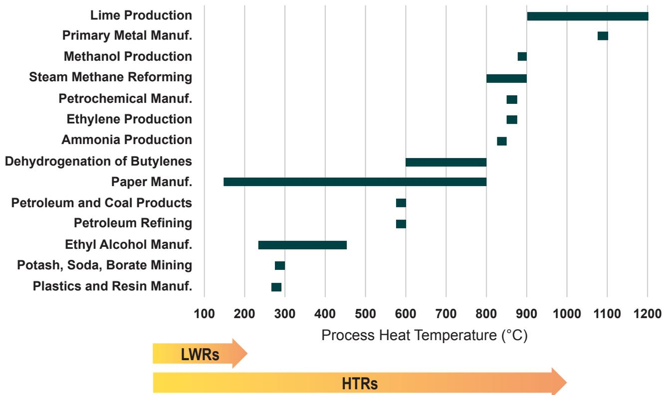
Figure 2: Potential process heat applications of CHP-enabled nuclear reactor IESs.
