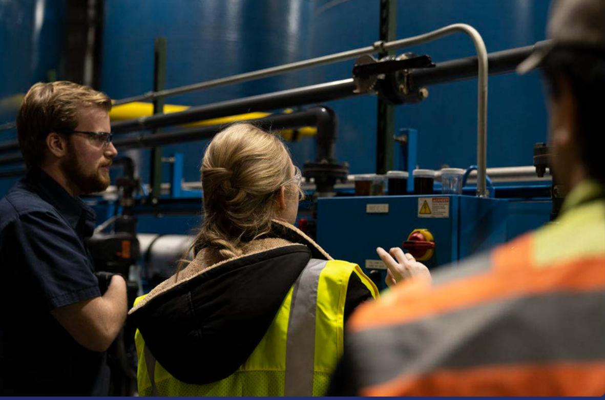
Fig. 2. The PFAS Annihilator by Revive Environmental, a Battelle company, is used to destroy PFAS through supercritical water oxidation. (Photo: Battelle)
