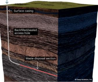
Technical diagram from Deep Isolation demonstrating a horizontal borehole disposal concept.
