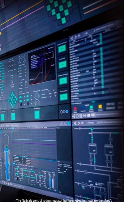
The NuScale control room simulator has been used to showcase the plant' design, prototype new displays, and test the operator and supervisor procedures in a fully digital control room. (Photos: NuScale Power)
