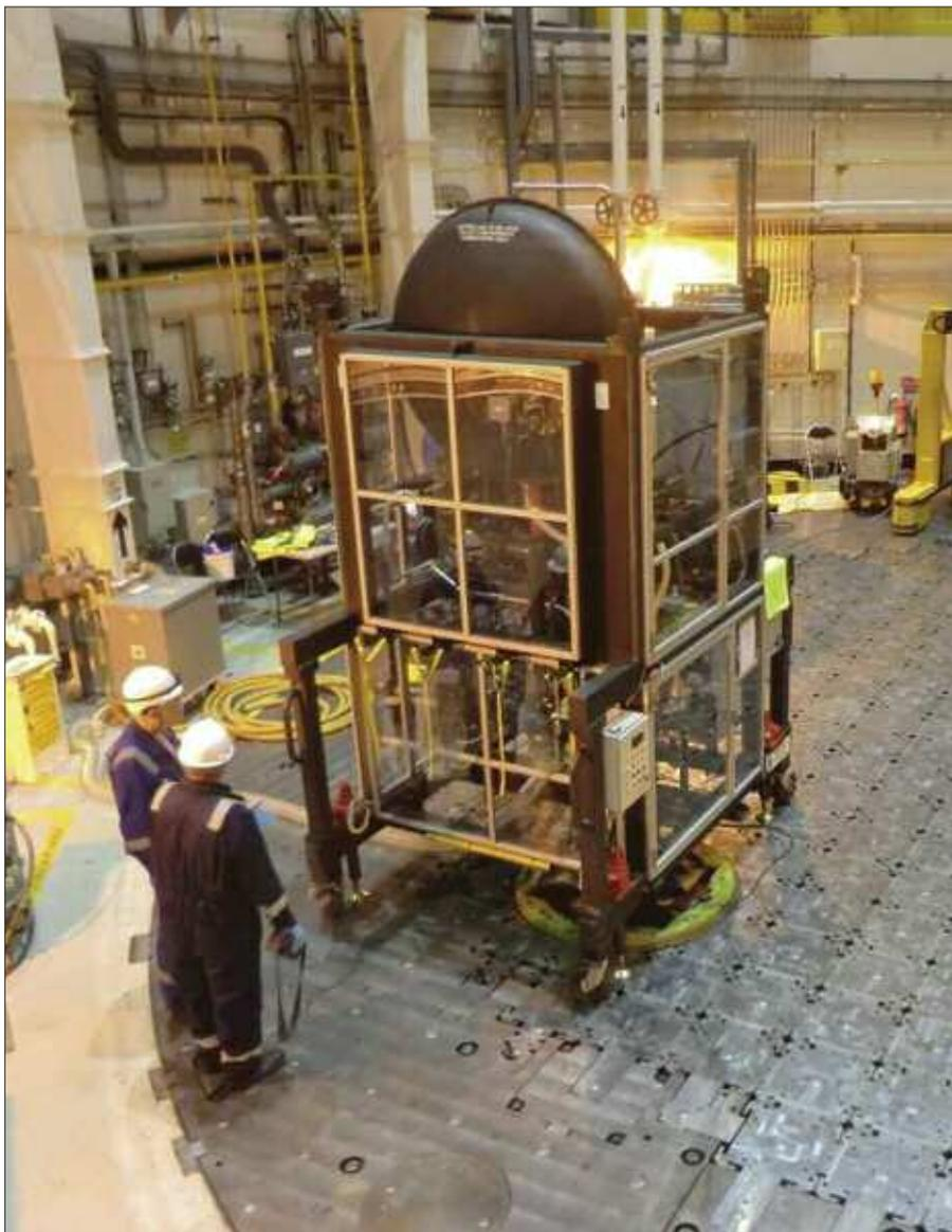
The graphite core channels in an advanced gas-cooled reactor are inspected by removing fuel assemblies from the top of the reactor and lowering inspection equipment down into the empty fuel channel. The New In Core Inspection Equipment (NICIE) tool allows for video inspection of the channel, looking for cracks in the graphite blocks and measuring both the bore profile and tilt of the channel, which check for swelling in the graphite.
