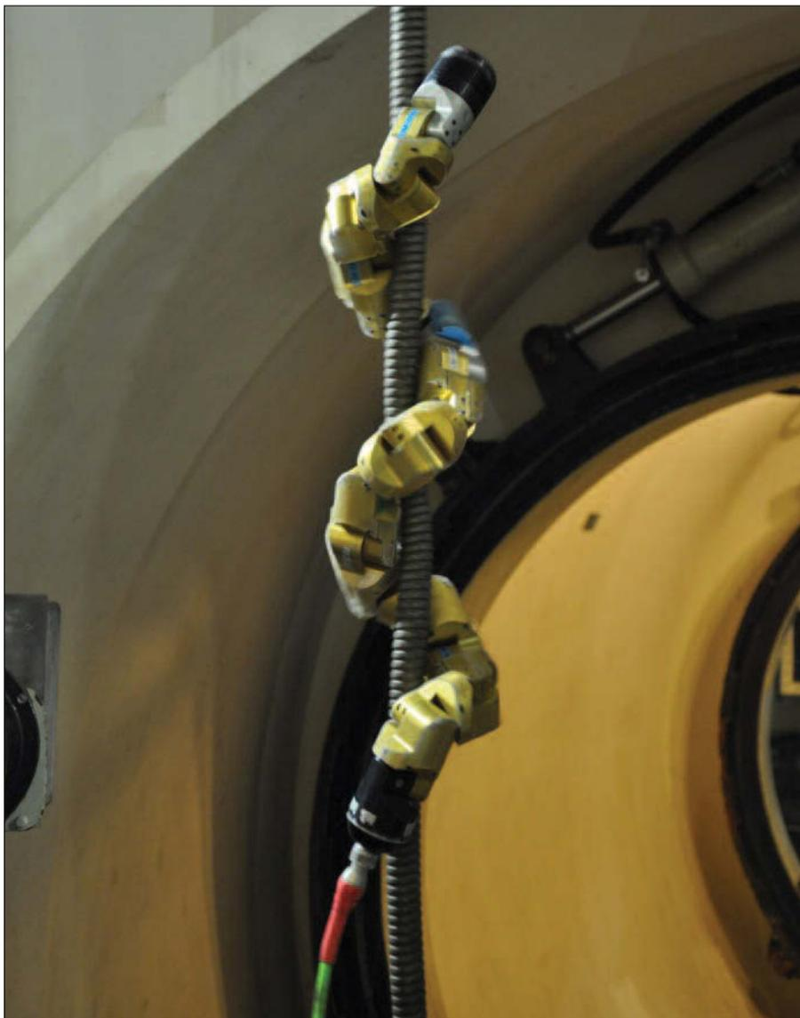
In a demonstration of its climbing capabilities, the snake robot climbs a cable at the Zwentendorf plant.
